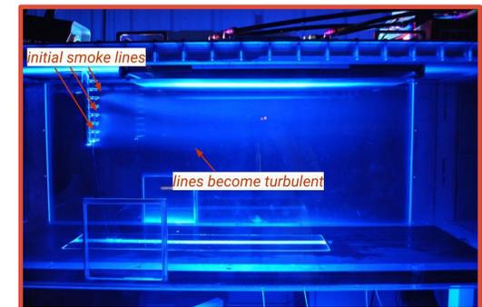
Fig. 3. Smoke trails developing under a flat metal plate.
