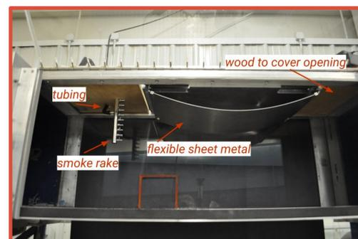
Fig. 2. The complete wind tunnel setup from the side.
