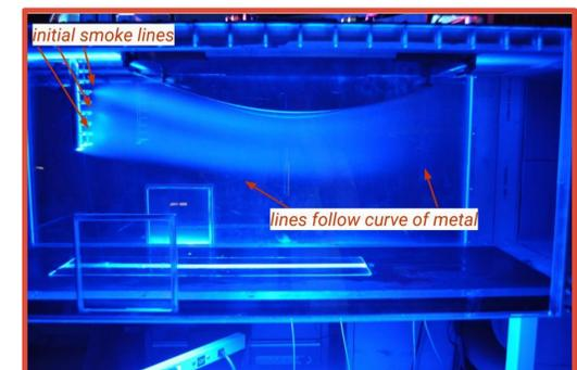
Fig. 4. Smoke trails developing under the same sheet metal, now curved.
