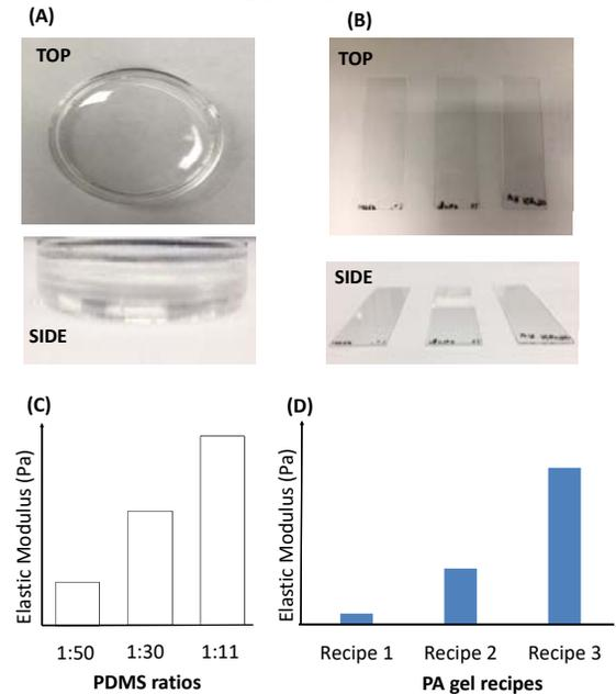
Figure 3 (A): Image of fabricated PDMS hydrogel (B): Image of fabricated PA hydrogel (C): Graph showing the elastic modulus of each PDMS curing/polymer ratio. D) Graph showing the elastic modulus of each PA recipe.
